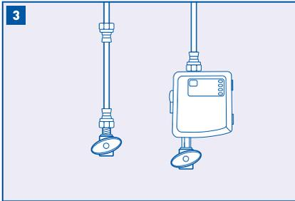
Tighten the control box to the cold water shut-off valve as shown. Tighten the lower end of cold water line onto the top of the control box.
