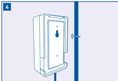
4 Use the provided screw to hang the battery box on the side of the cabinet.
