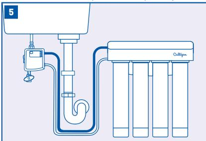
Connect the outlet on the RO/Filter system to the port marked "RO/Filter <." Wet the end of the plastic tubing with water and push it into the quick connect fitting adapter approximately 5/8" until it stops.
