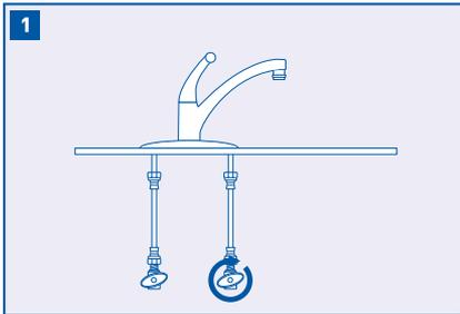
Turn off cold water shut-off valve then turn on the kitchen faucet and allow all water to drain from line.
