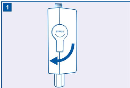
1 Confirm that the bypass valve is in the closed position (pointed down).
