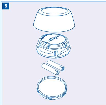
Install two AAA batteries (not included) into the remote button.
