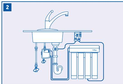
2 Turn on the cold water supply and check for leaks. If it leaks, refer to troubleshooting.
