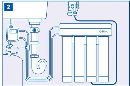
Connect the drain line coming from the RO system to the small connection of the air gap device.
