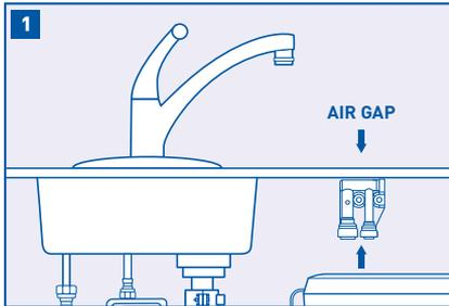
Mount the air gap device as near to counter top as possible and in a vertical orientation.
