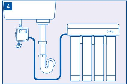
Connect the inlet on the RO/Filter system to the port marked "RO/Filter >." Wet the end of the plastic tubing with water and push it into the quick connect fitting adapter approximately 5/8" until it stops.
