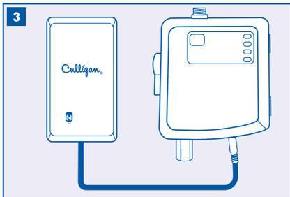
3 Install four C batteries (not included) into the battery box and plug into the jack on the bottom of the control box.
