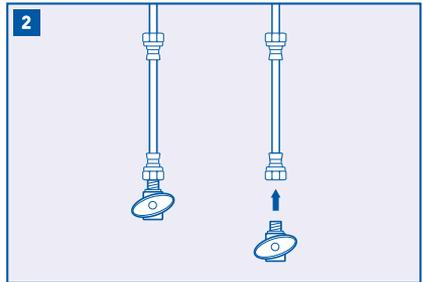
Disconnect the cold water line from the cold water shut-off valve.
