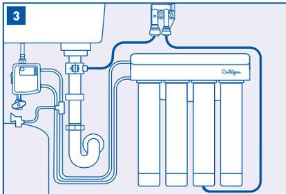
Connect the large fitting of the air gap device to the connection on the drain plumbing.
